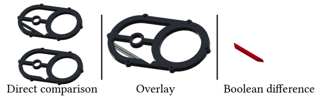
Figure 9: Instead of comparing side-by-side geometry (left), the user can overlay geometry and change their opacity (middle) or they can visualize the boolean difference (right).
